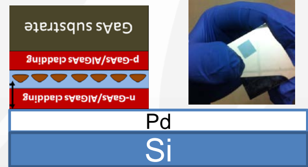
3) Flip-chip wafer bonding
